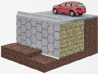
Reinforced Earth walls
